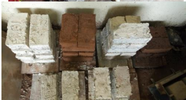
Plate 7: brick samples after production
