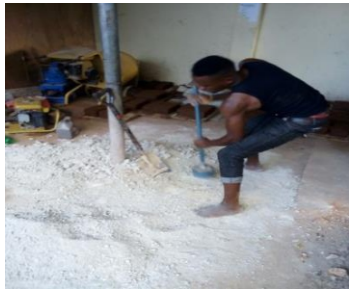
Plate 1: Breaking the clay lumps
