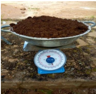
Plate 3: Batching of both soil samples
