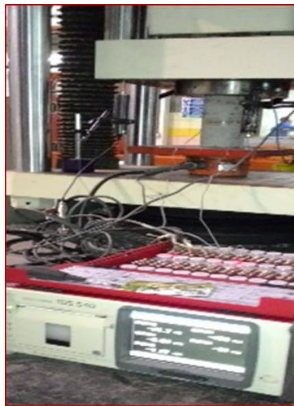
Figure 2. E-modulus test set-up
