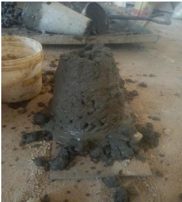
Figure 3: Sample undergoing slump test
