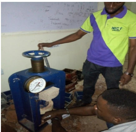
Plate 2: Compressive strength test
